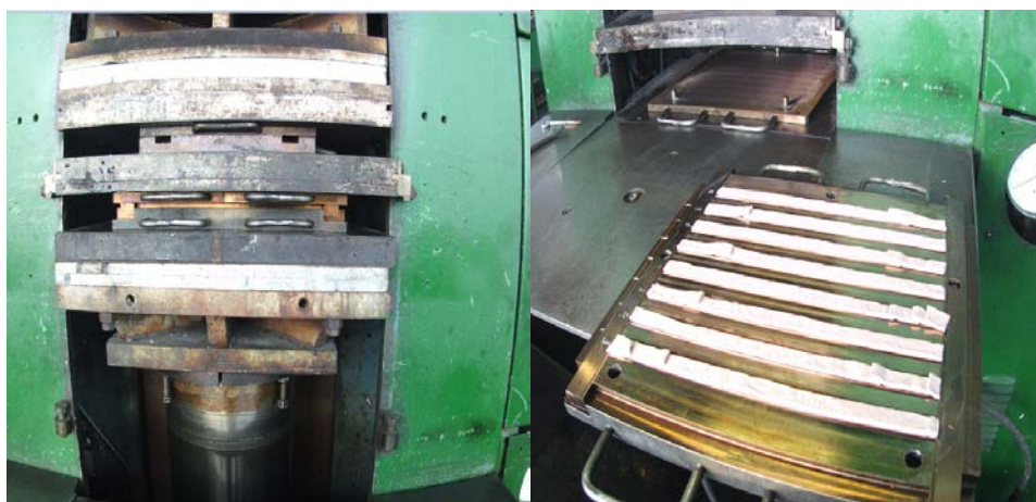
Fig. 1 – Work surface after processing of the SHS on a hydraulic vulcanizing press
